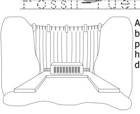
A **hydroelectric plant** also generates electricity by using a turbine to operate a generator that produces electricity, but instead of fossil fuels, a hydroelectric plant uses water stored behind a dam.
